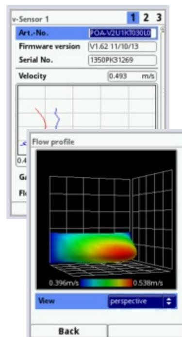
The NivuFlow 750 uses up to 9 x 16 gates for flow measurement. A flow profile can be directly indicated on the display.
