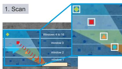
A few milliseconds later a second scan follows. The resulting echo patterns are saved as well.
