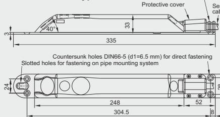
**Air-Ultrasonic Level Sensor, Type OCL**
