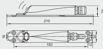
**Level sensor, Type DSM**
