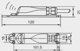
**Flow velocity sensor CSM-D**
